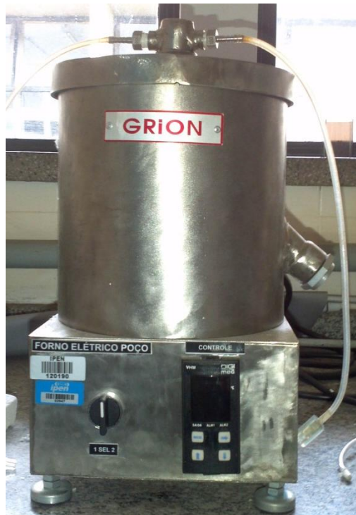
Figure 2: Furnace designed for \text{HgI}_2 crystals growth
