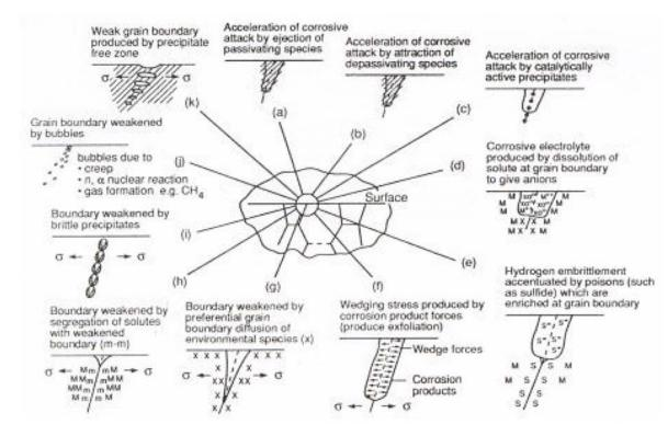
The processes starting from (a) to (k) range from the mostly chemical to the mostly mechanical (from R.W. Staehle, Combining design and corrosion for predicting life, in: R.N. Parkins (Ed.), Life Prediction of Corrodible Structures, vol. 1, NACE International, Houston, 1994, pp. 138–291)
