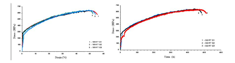
Alloy 600 MA specimens stress-strain curves. SSRT 01 (neutral environment of  $N_2$ ), SSRT 02 and 03 (PW environment at 303 °C and 10 MPa). Initial strain rate of 3,0x10<sup>-7</sup>s<sup>-1</sup>
