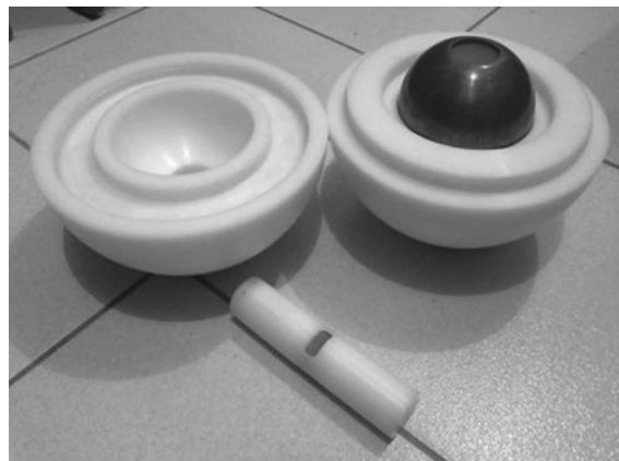
Fig. 4. Passive dosimetric system, based on CR39 PADC in polyethylene/lead sphere.
