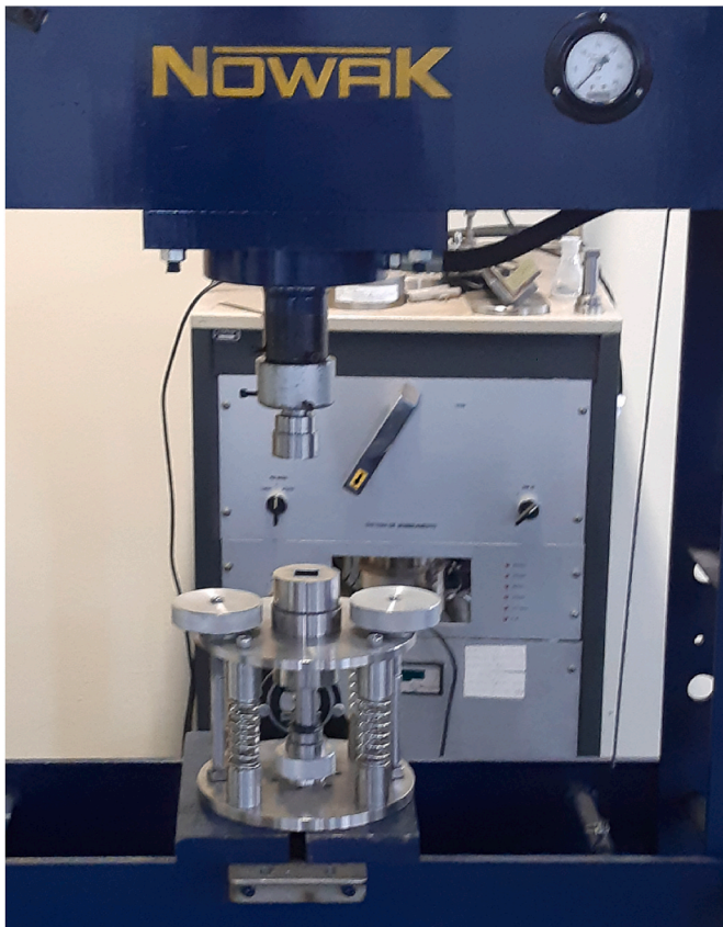
Fig. 6. Pressing system showing the floating die.
