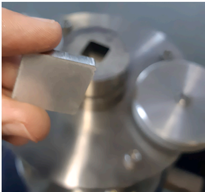
Fig. 7. Photograph depicting a representative B 4 C-Al briquette.
