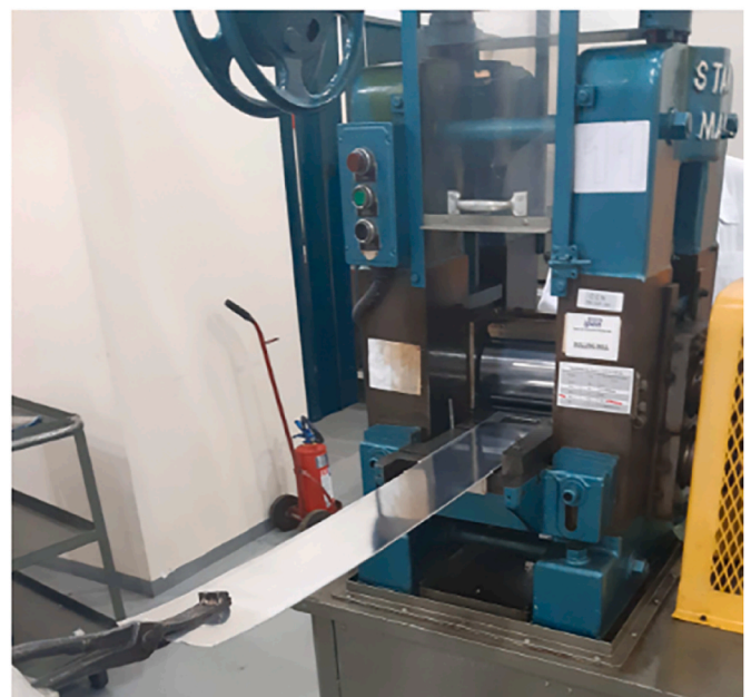
Fig. 9. Rolling process for the absorber plates.
