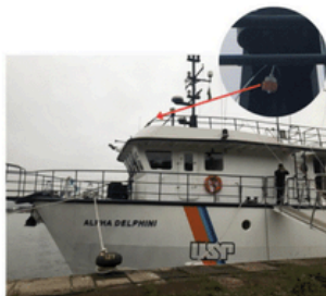
Figure 2. Vessel Alpha Delphini IOUSP, in destak the position inlet of portable gas analyzer
