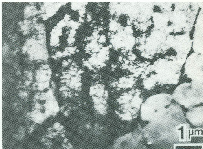
Fig.11 - TEM micrograph of 7050 RS Al alloy; cellular array where a low density of precipitates inside the cells is present (the precipitation occurs preferentially at the boundaries).
