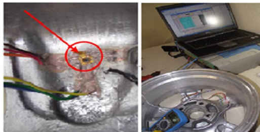
Figure 4 - Hole drilling gages rosette
