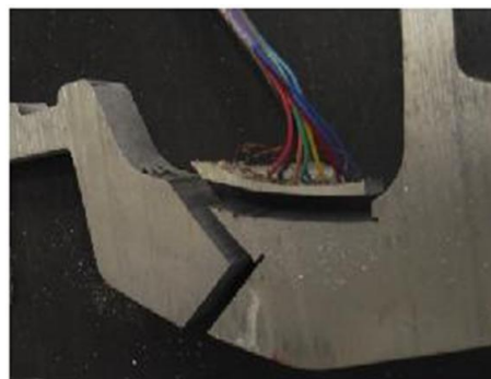
Figure 5 - Minimal section for hole drilling method
