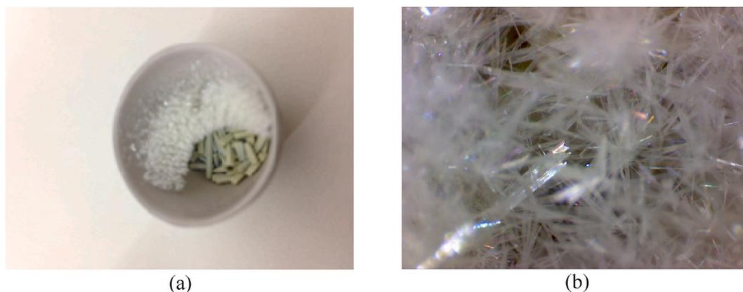
Fig. 9. RTT-1 processing on spent HCC catalyst from lower zone: a) alumina crucible and b) crystal formed after electron beam irradiation.
