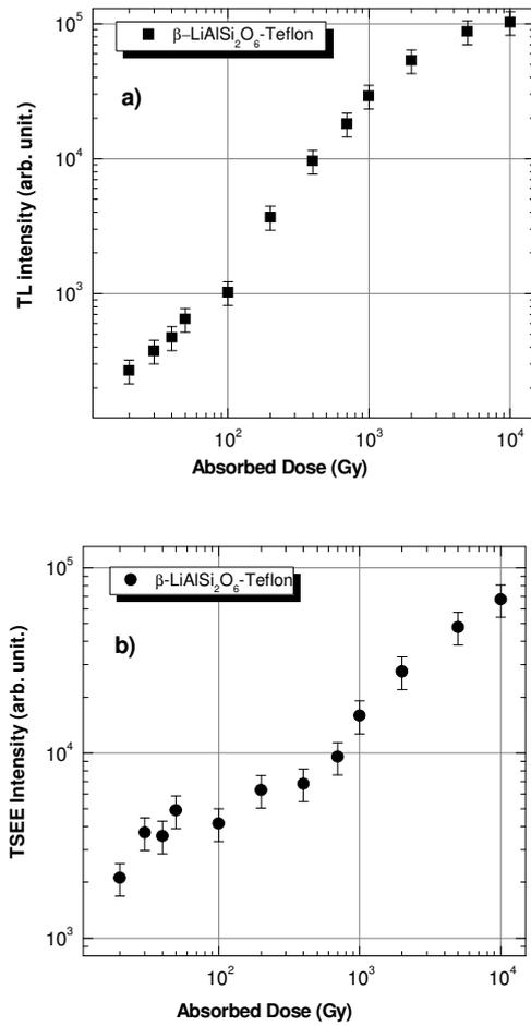
**Fig. 3.** TL (a) and TSEE (b) dose-response curves of  $\beta$ -spodumene-Teflon® pellets irradiated with the <sup>60</sup>Co source.
