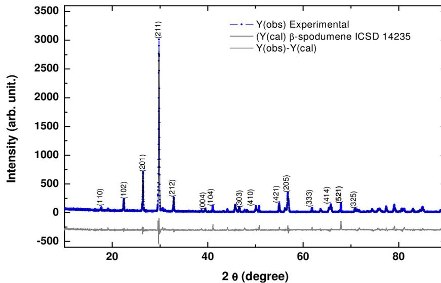
**Fig. 1.** X-ray diffraction pattern of a powder sample of pure synthetic spodumene  $Y(obs)$  compared with the calculated spectrum by the Rietveld method  $Y(cal)$ . The result of refinement is shown by the difference  $Y(obs) - Y(cal)$
