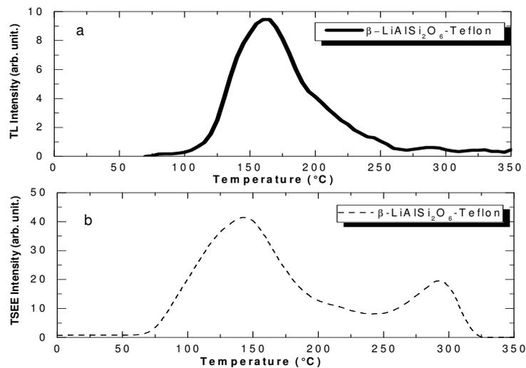
**Fig. 2.** TL (a) and TSEE (b) emission curves of  $\beta$ -spodumene-Teflon® pellets irradiated with 50 Gy ( $^{60}\text{Co}$  source) at room temperature.
