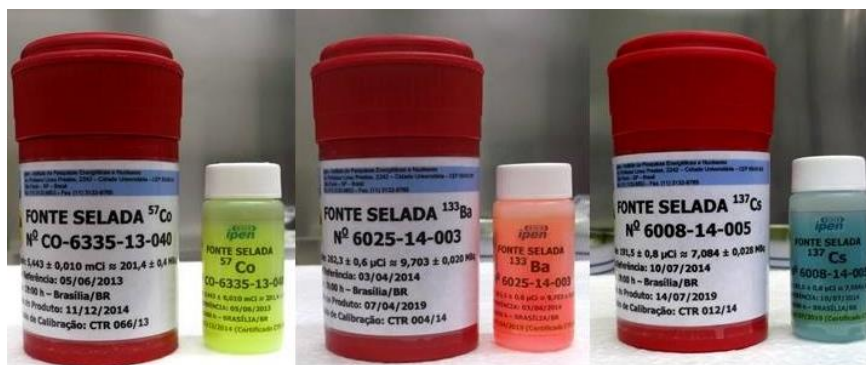
Figure 2: Sealed radioactive sources produced with cobalt-57, barium-133 and cesium-137. Made at the Institute of Energy and Nuclear Research (IPEN).
