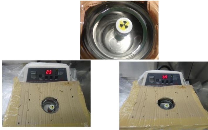
Figure 4 : Source immersed for leaking tests.
