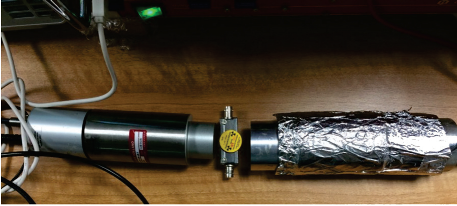
Fig. 93. The setup employed for energy and time resolution of the gamma CALORIMETER by using a V1782 digitizer (100 MS/s). Two scintillators, coupled to photomultipliers, were placed face to face with a ^{22}\text{Na} \beta^+ source in between producing two back-to-back gamma rays of 511 keV energy and a single one of 1274 keV. On the left a CeBr scintillator, on the right a LaBr 3 scintillator.
