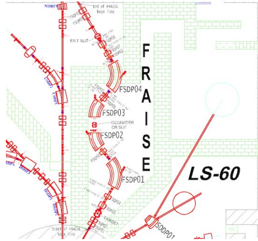
Fig. 6. Layout of the FRAISE beam line, that will be used to select the energy spread and the beam emittance size to match the NUMEN experiment request.
