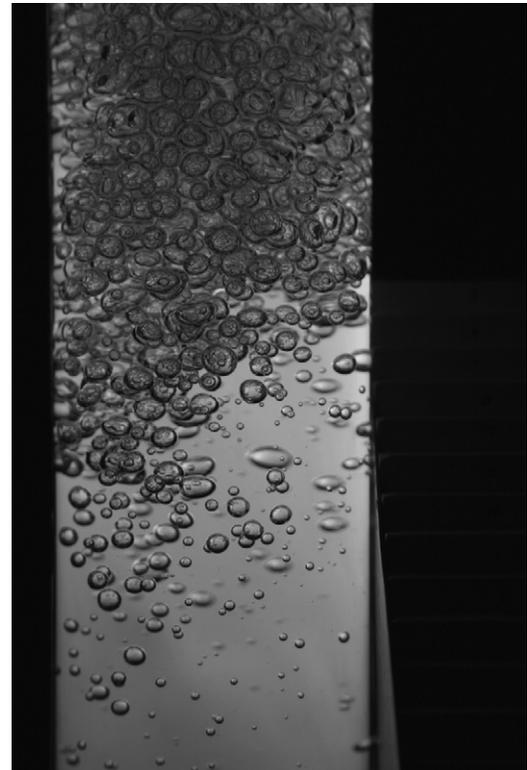
Fig. 5. Characteristic image of periodic transition from refill-to-incubation phase in ascending flow of a chugging instability.
