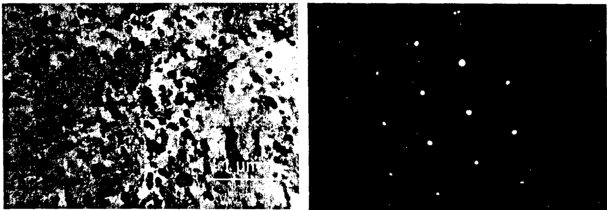
Figure 3 (a–b). Transmission electron micrograph of the forged and thermally treated (835°C for 1 hour) material: a) fine precipitates inside grains, b) selected area diffraction pattern (SAD); precipitates are \text{Ni}_3\text{Mo} and \text{Ni}_3\text{Ti} types.
