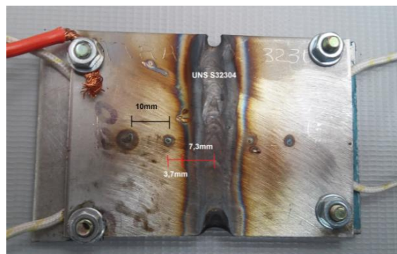
Figure 3. Welded sample plate showing thermocouples positions and distances from the weld bead.
