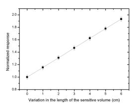
Figure 4 - Linearity of response to the variation of the sensitive volume length.
