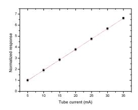
Figure 3 - Linearity of response with the X ray tube current variation
