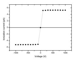
Figure 2 - Saturation curve obtained of the free air ionization chamber in the collapsed position for the voltage in both polarities. The maximum uncertainty of the measurements was 0.5%, not visible in the graph.
