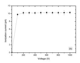
Figure 1 - Saturation curves of the free air ionization chamber in the (a) collapsed position; (b) expanded position.
