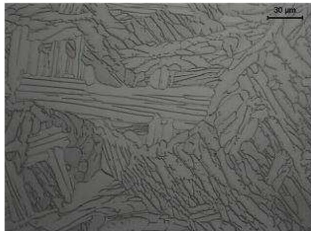
Fig. 2. Ti-6Al-4V alloy micrograph of Widmanstätten structure.
