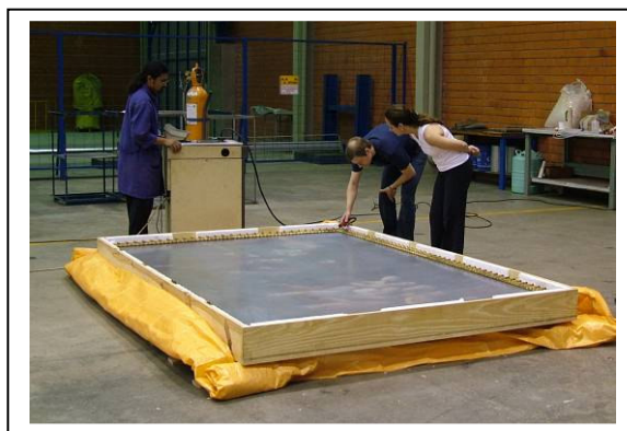
Figure 3. Checking the leakage of helium gas from the acrylic box by a Sniffer probe.
