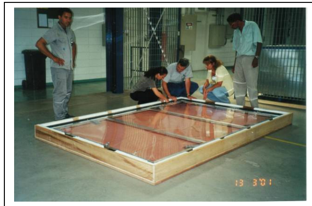
Figure 2. The back side of the painting with acrylic protection inside of the wood box lined with expanded polystyrene being observed before the first irradiation.
