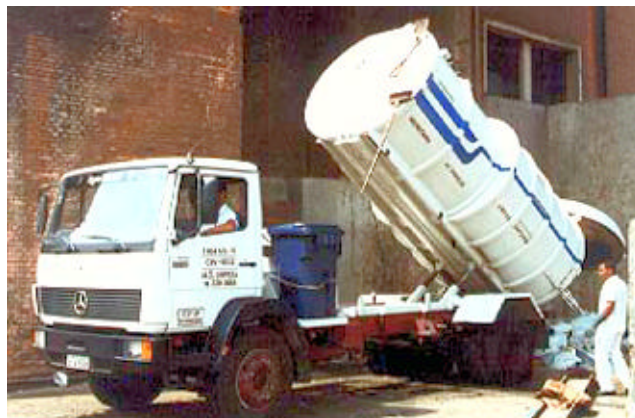
Figure 2. Collecting Truck Being Unloaded.
