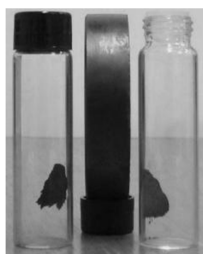
Figure 1. Magnetic responses of the ZM3 (left) and ZC2 (right) in contact with a magnet.
