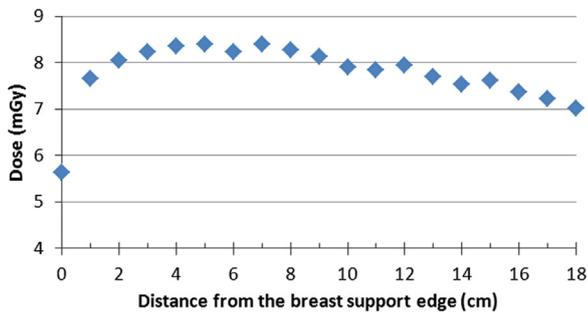
Fig. 3. Variation of the radiation intensity along the breast support. At distance zero the attenuation caused by the beam collimation reduces the patient's chest wall dose.
