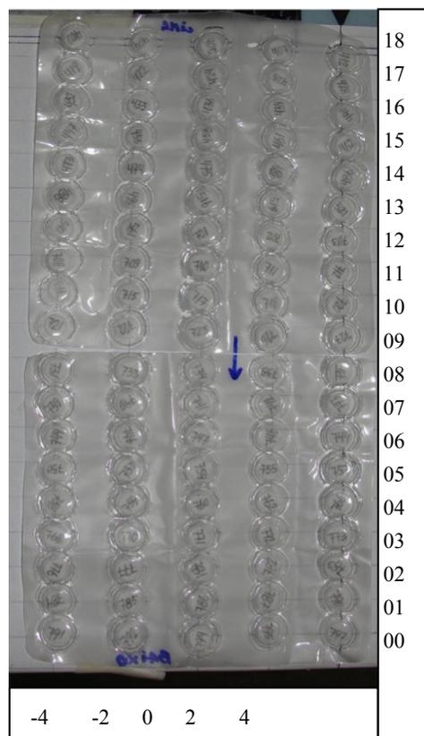
Fig. 2. TLDs distribution matrix used in the mammography system mapping.
