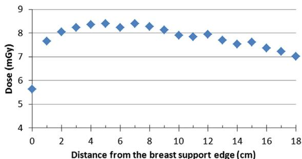
Fig. 3. Variation of the radiation intensity along the breast support. At distance zero the attenuation caused by the beam collimation reduces the patient's chest wall dose.
