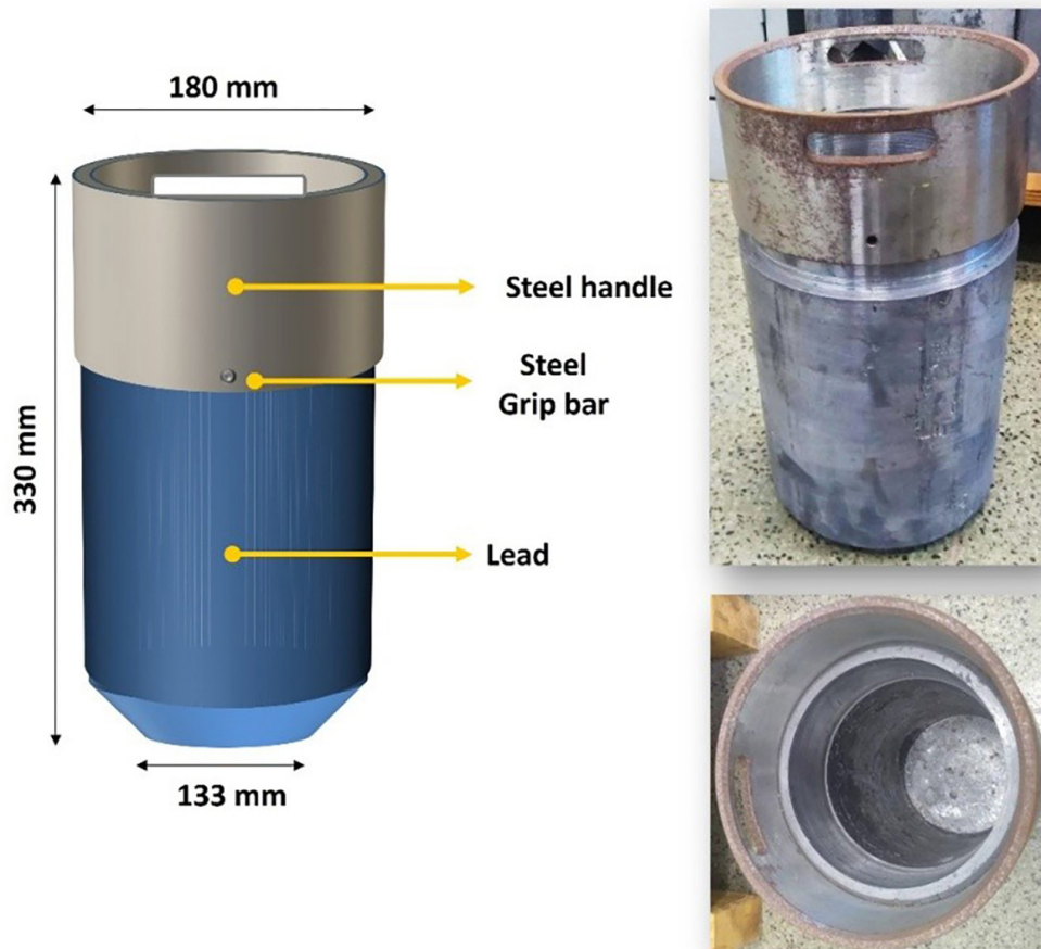
Figure 7: Brazilian proposed borehole container concept. Based on [23].
