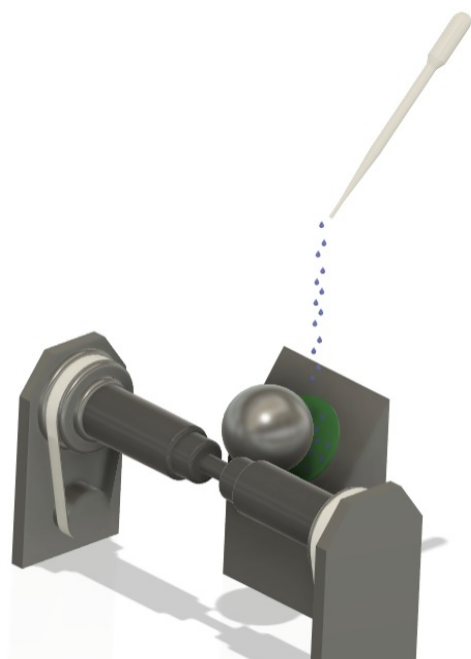
Figure 1. Three-dimensional schematic representation of the operational principle of the ball-cratering tribological test.
