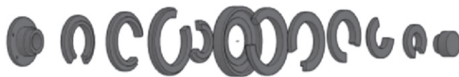
Figure 1. Exploded view of the truncated rings which compose the collimating set used in the experiment.
