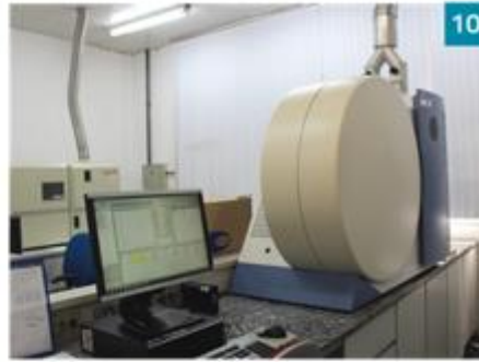
Argon plasma optical emission spectrometry (ICP-OES)
