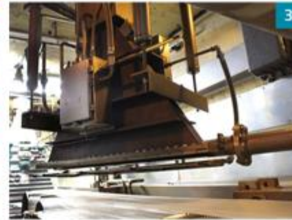
3 1.5 Mev electron accelerator and 65mA beam
