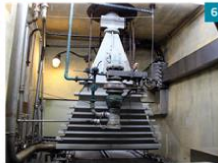
6 1.5 Mev electron accelerator and 25mA beam
