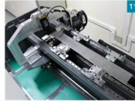
Automatic machine for measuring combustible plates by laser triangulation
