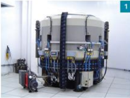
1 Cyclone 18 - 18Mev cyclotron particle accelerator
