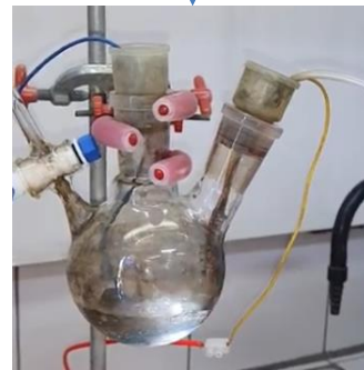
Synthesis of high purity graphene by bottom-up process
