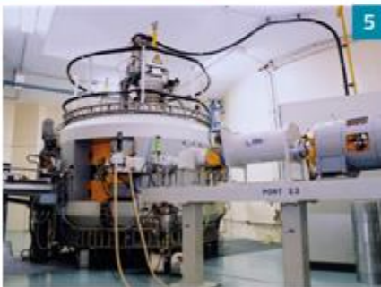
5 Cyclone 30 - 30 Mev particle accelerator
