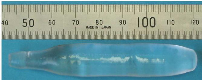
**Fig. 2: Czochralski grown scheelite mixed crystal  $\text{Li}(\text{Lu}_{0.75}\text{Gd}_{0.25})\text{F}_4$ .**
