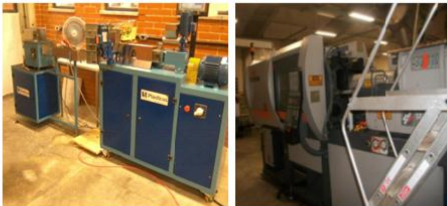
Figure 1: On the left the "AX 16LD40" Extruder and on the right the "430/110" Injection molding machine
