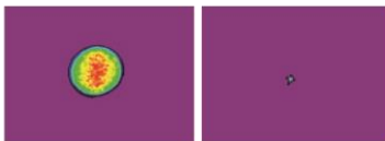
Near field @532 nm, Stable resonator Far field @532 nm, GRM
