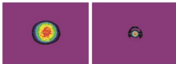
Near field @1064 nm, Stable resonator Far field @1064 nm, GRM resonator
