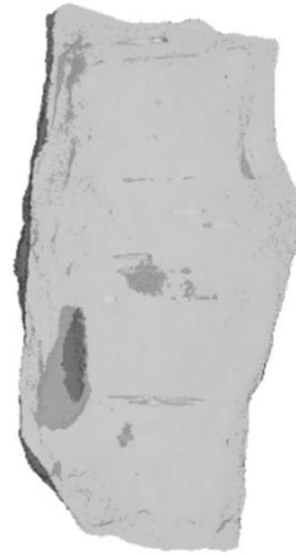
Fig. 9 Tomography of the dry tile at 0^\circ
