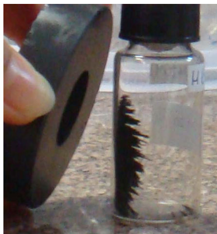
Figure 1. Magnetite powder obtained from the reaction of Fe ^{2+} ions and OH ^{-} ions, exposed in magnet field of a magnet.
