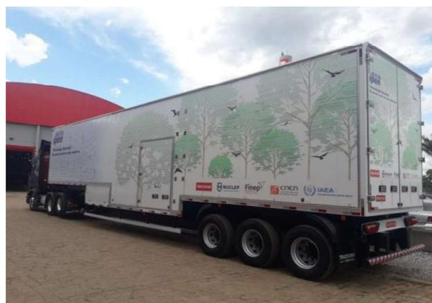
**Fig. 5.** Mobile Unit (0.7 MeV and 20 kW) developed by IPEN-CNEN/SP.
