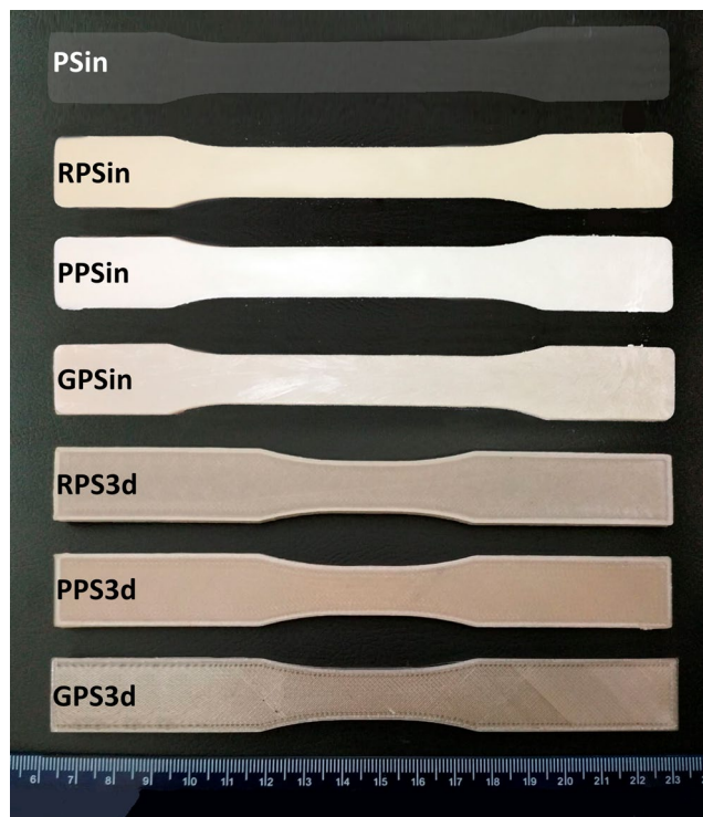
Fig. 1 Specimens of injected samples: expanded polystyrene recycled with glycerol and 10 wt% gypsum (GPSin); expanded polystyrene recycled with 2 wt% glycerol as plasticizer (PPSin). Specimens of 3D printed samples: GPS3d; PPS3d; expanded polystyrene recycled without glycerol (RPS3d)
