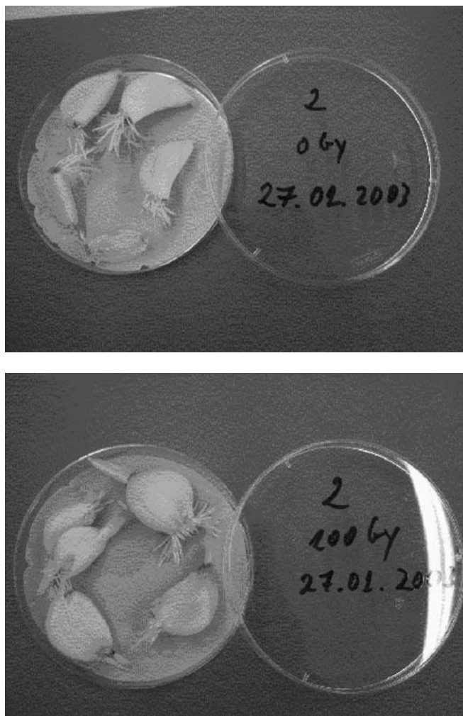
Fig. 3 Germination tests for garlic samples (code 2) from the German market (samples with codes 1, 3 and 4 look similar)
