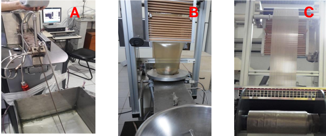
Fig.1 - Polypropylene nanocomposite blend in the extruder with spaghetti training "masterbathes" (A); Haake film blowing unit used to prepare the blown films (B); The blown film take-off transports the extruded film in an upward direction. The film is guided up to the nip rolls where the tube is flattened to create a "lay-flat" tube of film (C).
