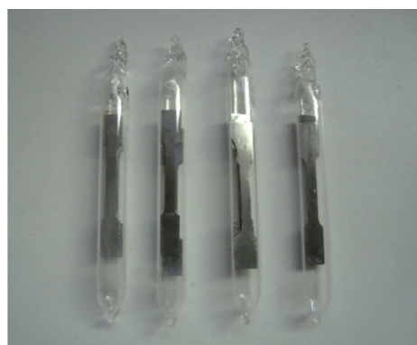
Fig. 3 – Cylindrical and prismatic specimens encapsulated in quartz glass for heat treatment.
