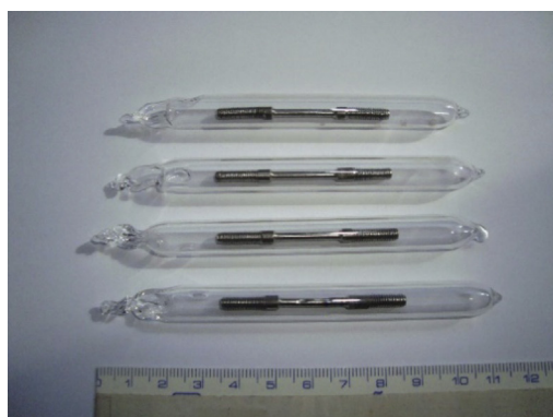
Fig. 3 – Cylindrical and prismatic specimens encapsulated in quartz glass for heat treatment.
