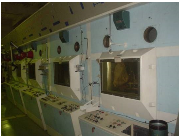
Figure 2 - CELESTE Project hot cells. Source: [8]
