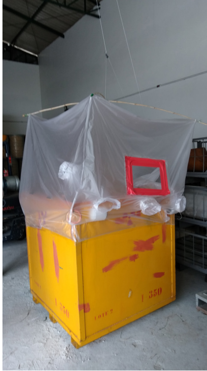
Figure 1 - Plastic cap over the waste box.
