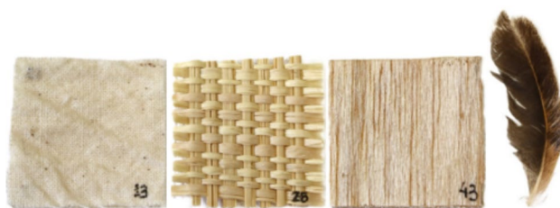
Fig. 2 From left to right: mock-ups made of cotton, vegetable fiber, wood, and feathers contaminated with pesticides. The figure is not to scale; actual sample dimensions are provided in the description above
