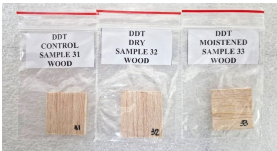
Fig. 3 Batch of wood mock-ups contaminated with 10.0 ppm DDT, separated into the three experimental conditions: a control, b dry and c moistened
