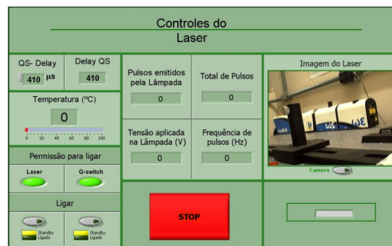
Fig. 2. Laser control front panel VI layout.
