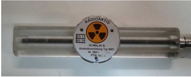
Fig. 4. Radioactive check source positioned at the special acrylic support into which the CT ionization chamber was inserted.
