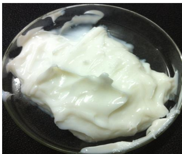
Figure 1: Polyurea grease obtained by reaction of long chain monoamine, short chain diamine and an aromatic diisocyanate.
