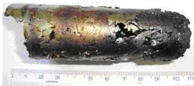
Fig. 1 Ingot of remelted Zircaloy obtained by VAR process
