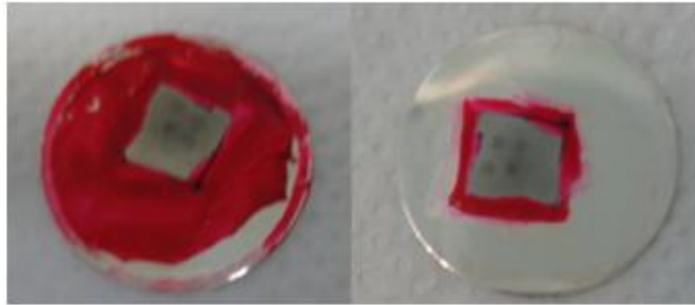
Figure 5: Americium electrodeposited source with and without red nail polish
