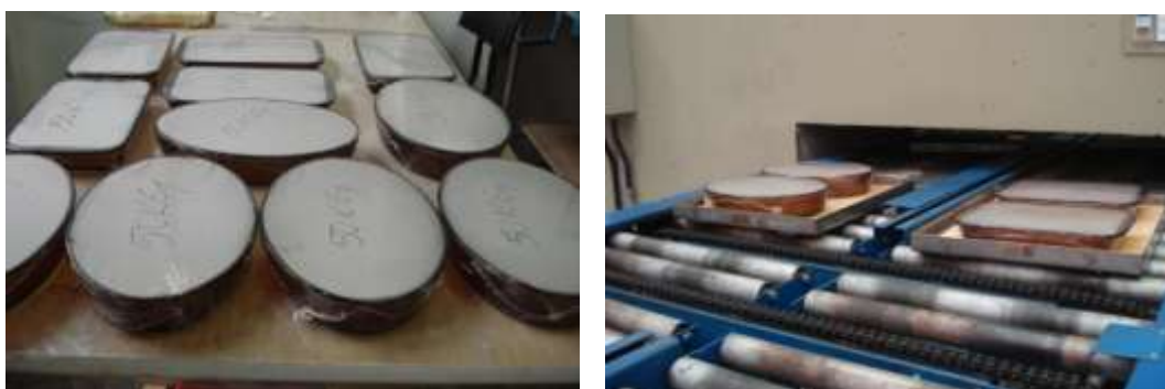
Figure 1. Samples prepared for electron beam irradiation
