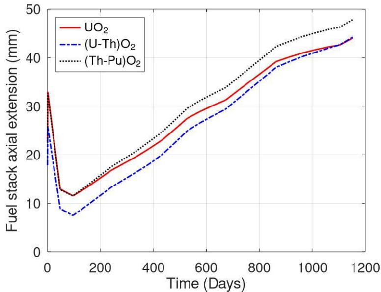
Figure 2. Fuel stack elongation under the burn cycle for UO<sub>2</sub>, (Th-U)O<sub>2</sub>, and (Th-Pu)O<sub>2</sub>.
