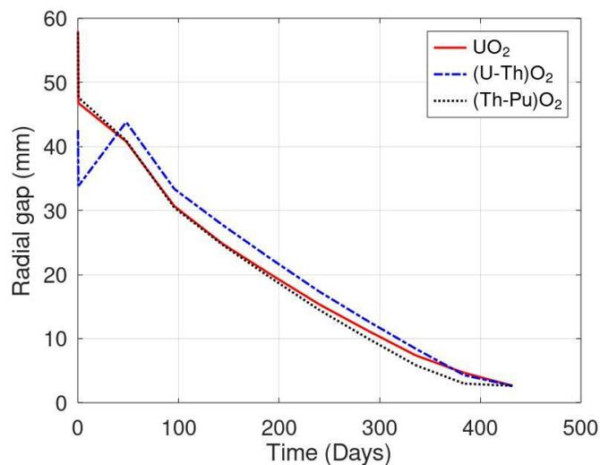
Figure 3. Radial gap space during the burn cycle for UO<sub>2</sub>, (Th-U)O<sub>2</sub>, and (Th-Pu)O<sub>2</sub>.
