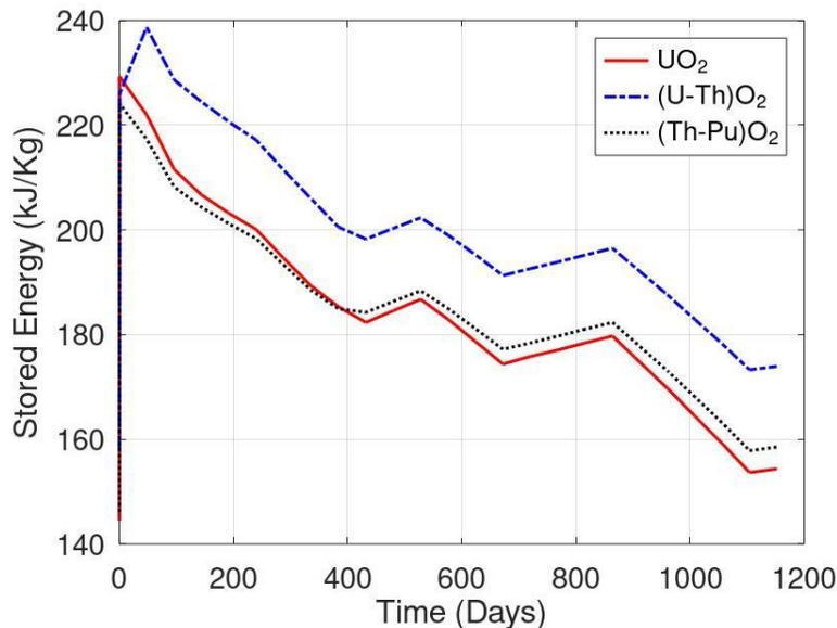
Figure 4. Stored energy during the burn cycle for UO<sub>2</sub>, (Th-U)O<sub>2</sub>, and (Th-Pu)O<sub>2</sub>.
