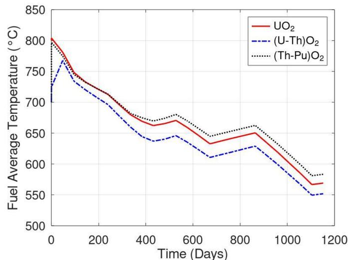
Figure 1. Fuel temperature in the burn cycle for UO<sub>2</sub>, (Th-U)O<sub>2</sub>, and (Th-Pu)O<sub>2</sub>.
