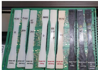
Figure 1: Non-irradiated and irradiated A, B and C polyethylene specimens (100 kGy and 300 kGy doses) before going through the lead-free reflow soldering.
