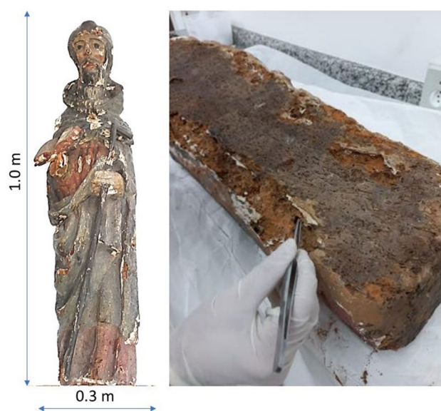
Fig. 1 Wooden sculpture of Saint Jerome. Severely degraded, internal porosity and weak structure
