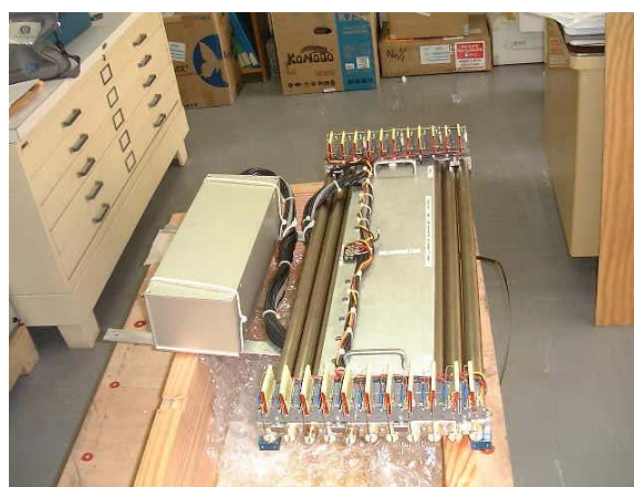
FIGURE 4. Back view of the PSD array. Preamplifiers are identified by the large yellow capacitors at each end of the detectors. On the left of the detector is the Junction Box.
