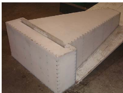
FIGURE 6. The detector shield ready to be installed in the diffractometer
