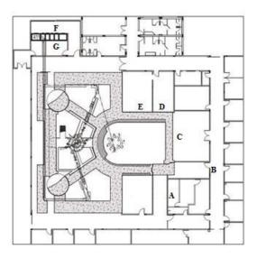
**Fig. 1.** Plant of the facility and the location of the monitored spots from A to E both gamma and neutron radiation are monitored. At F and G Spots, only gamma radiation is monitored
