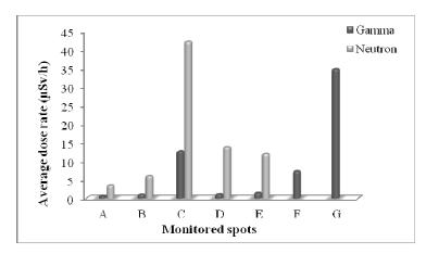
Fig. 3. Average dose rate for gamma and neutron radiation for each monitored spot
