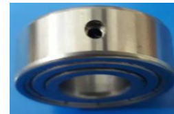
Fig. 4. Bearing with induced fault (hole) in the outer race
