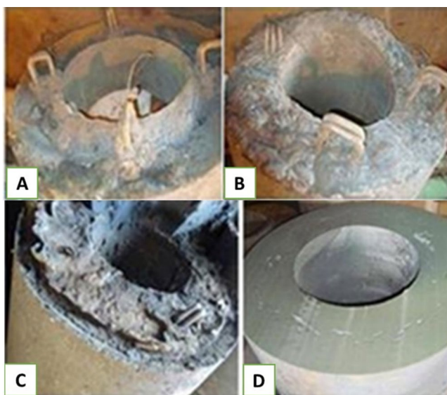
Fig. 2 Mill roller shells showing a riser without defect (A) and expanded riser (B and C). Mill sleeve with the riser removed, displaying a secondary shrinkage defect (D)
