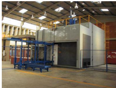
Figure 1: Compact Multipurpose Irradiator from IPEN / CNEN-SP.
